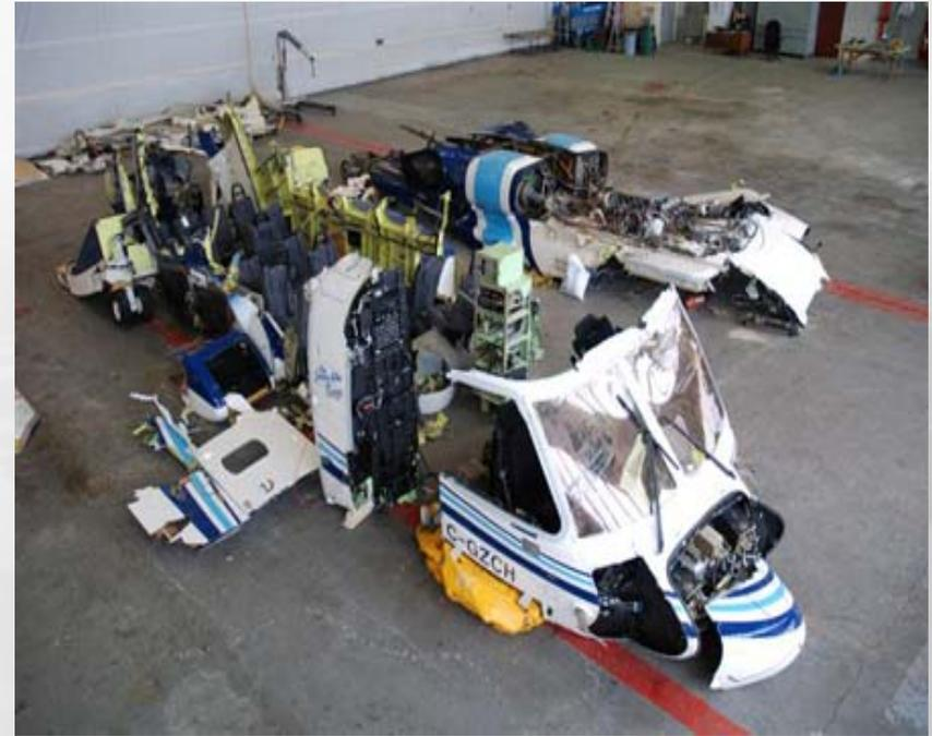
Wreckage layout and reconstruction (photo: TSB)
