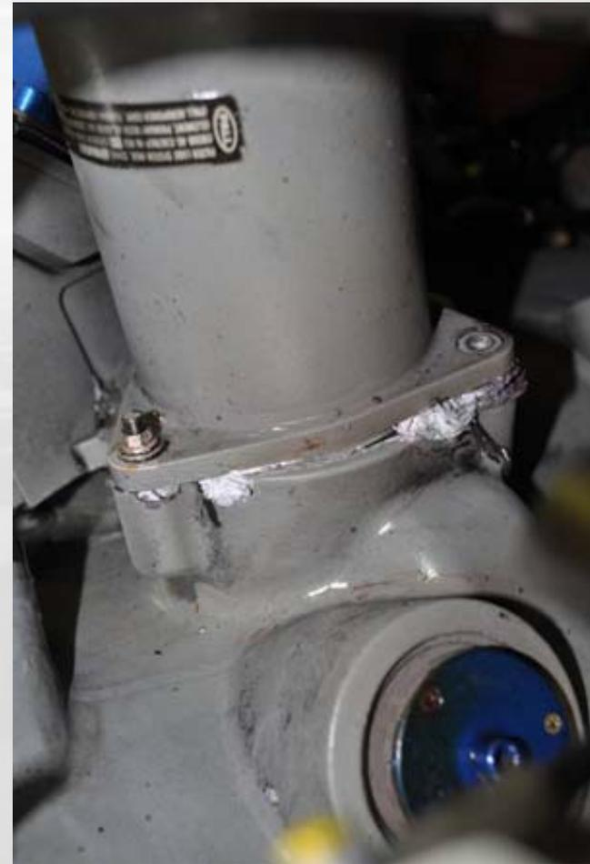
Oil filter housing showing broken and missing mounting stud (photo: TSB)
