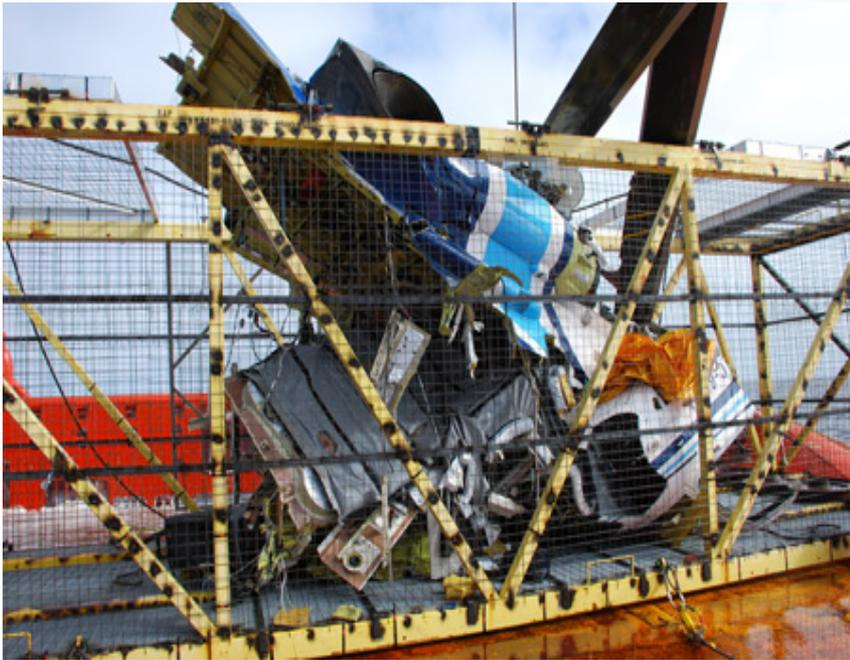
Right side of the 'upper deck' and fuselage structure (photo: TSB)
