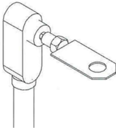
**Figure 6-7 Example of an LB Fitting and Plate Connection**
