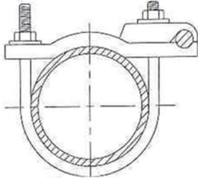
**Figure 6-3 Example of a Certified Ground Clamp Connection**
