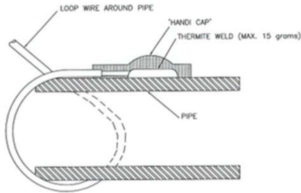
**Figure 6-4 Example of a Exothermic Weld Connection**
