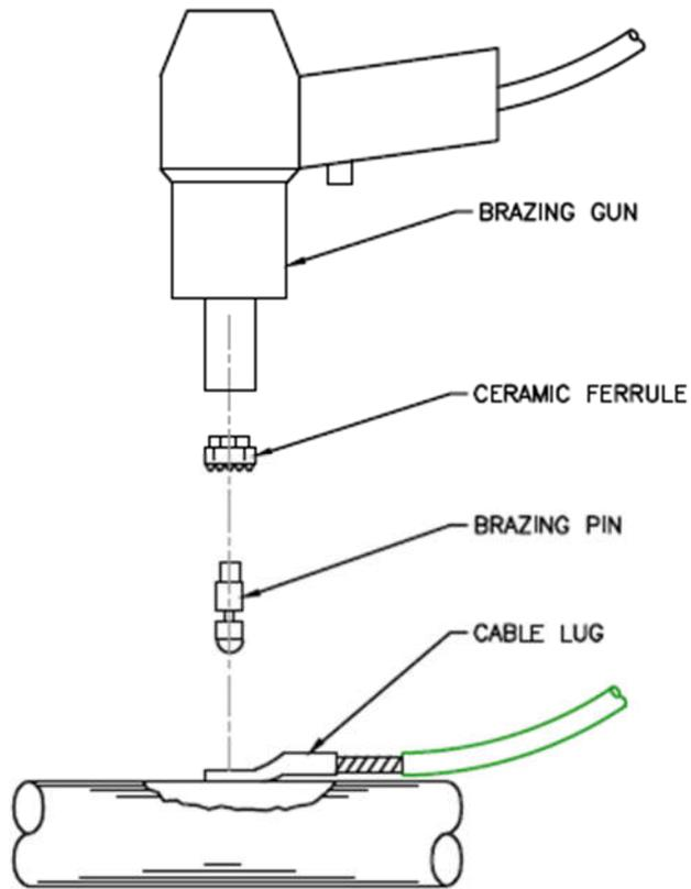
Figure 6-5 Capacitive Discharge Stud Welding System.
