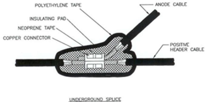
Figure 7-1 Example of a Splice Connection
