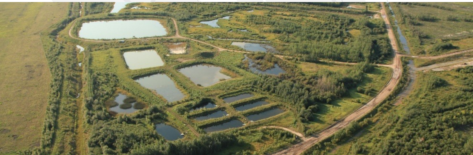
Pit lake (water-capped tailings technology) test ponds. (Photo credit Syncrude Canada Ltd.)
