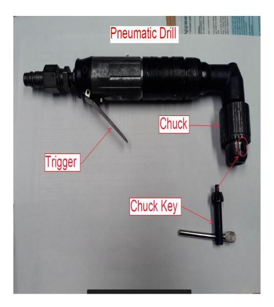
Picture 2 - Pneumatic drill with key inserted into chuck to remove/install drill bit
