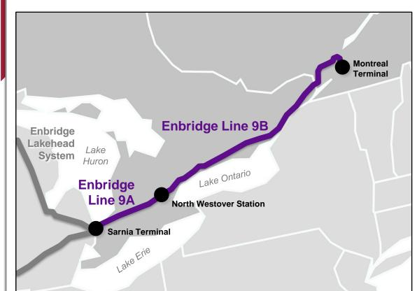
The Enbridge's Line 9 pipeline connects refineries in Sarnia to Montreal. The flow of oil through the pipeline has been reversed multiple times.
