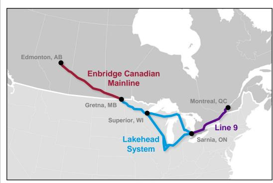
Originating in Edmonton, Alberta, the Enbridge Mainline moves crude oil, refined products, and natural gas liquids through a connected pipeline system. At Superior, Wisconsin, the system splits into Line 5, going north of Lake Michigan, and Lines 6, 14, and 61, going around the southern tip of the lake. The two routes then coalesce and terminate in Sarnia, Ontario, where it is interconnected with Line 9, which is terminated in Montreal, Quebec.
