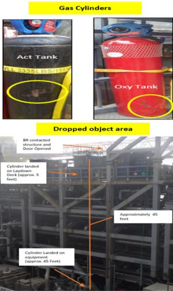
Fig. 2. Images of cylinders damaged during the incident and dropped object area
